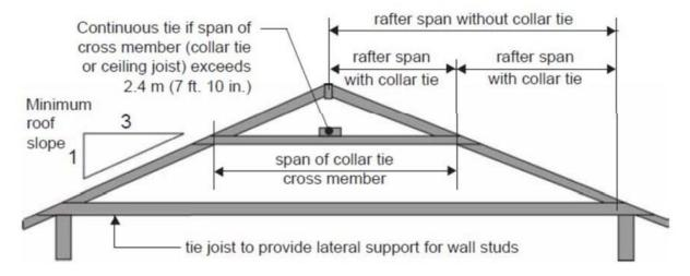
Table 6: Roof Rafter Spans — Rafter NOT SUPPORTING Ceiling
