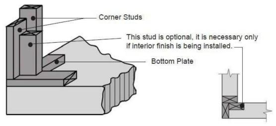
Figure 9: Exterior Wall Framing at Gable End Detail
