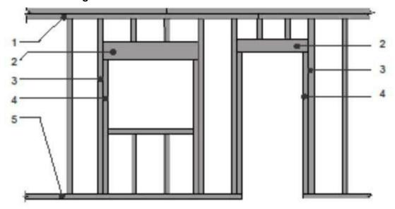
Figure 7: Wall Framing and Lintel Detail
