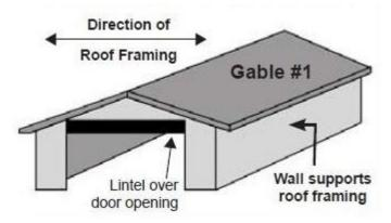
Table 4: Wood Lintels - NOT SUPPORTING Roof Loads
