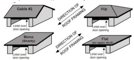
Figure 11: Roof Styles with Lintel Support Roof Framing
